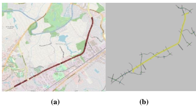
Figure 3: The Mainline Route chosen for the Study (a) Field ERV GPS data along the mainline overlaid on OpenStreetMap™ [36], (b) Mainline ERV Route Static Routing Decision in VISSIM®
